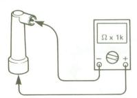
• Check the spark plug cap for specificated resistance.
