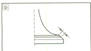
D Valve seat is too narrow and is located down near the bottom edge of the valve face.
