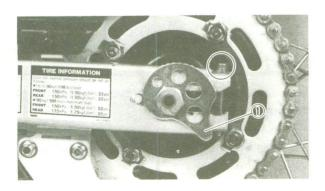
Turn the chain puller 1 clockwise or counterclockwise until the specified slack is obtained.
