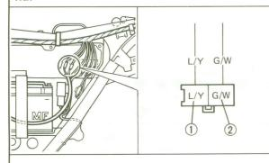
• Check the pickup coil for specified resistance.
