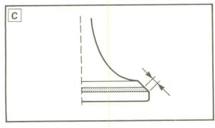
C Valve seat is too narrow and right up near valve margin.
