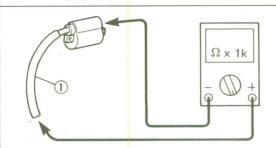
Check the secondary coil for specificated resistance.
