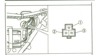
• Check the stator coil for specified resistance.
