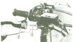
Install the brake hose as shown.
