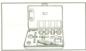
7. Valve seat cutter set P/N. YM-91043
