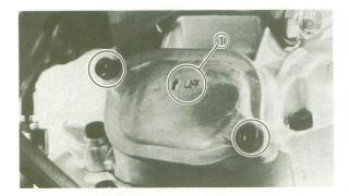
The tappet cover (intake) should be installed with the arrow mark (1) upward.
