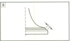
B Valve seat is in the middle of the valve face but too narrow.
