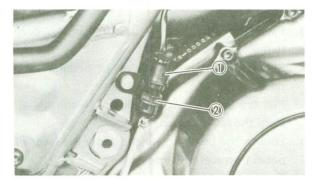
1. Hold the switch body ① with your hand so that it does not rotate and turn the adjusting nut ②.
