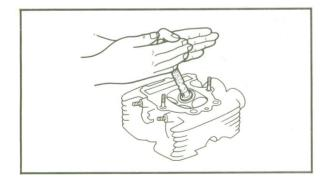
Turn the valve until the valve face and valve seat are evenly polished, then clean off all compound.
