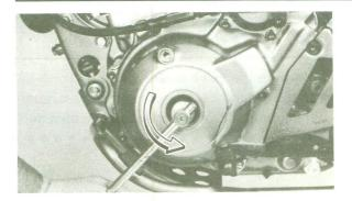
6. Turn the crankshaft counterclockwise with a wrench.
